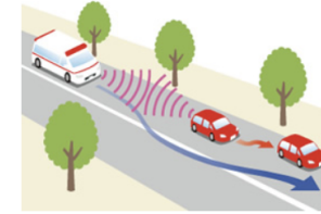
Assistance in Confirmation of Nearby Vehicles Assists in confirming vehicles in the vicinity using information from other cars
